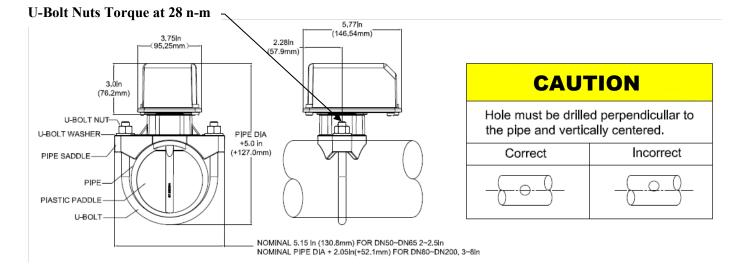
NOTE: Please make sure the SADDLE GASKET on the correction direction before installation.
