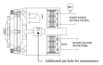
This additional pin hole would allow the wrench (coming with the device) to insert into it and temporarily stop the device from functioning causing false alarm during the maintenance. When the wrench is in there, it also prevents the red device cover to be re-installed.
