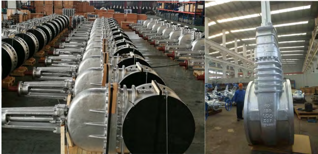
30"-150 GATE VALVE in mass production
