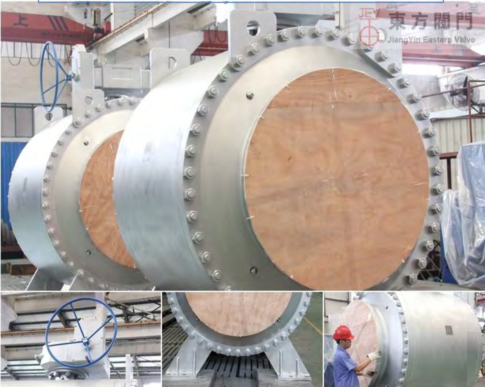
Floating Ball valve available for subsea PTFE coating
