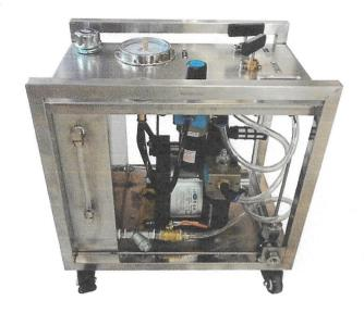
After the cylinder is filled with water, the hydraulic pressure test is carried out. The water pressure test machine pressurization device is connected to the bottle, and the pressure is increased to the pressure required for hydrostatic pressure testing.
